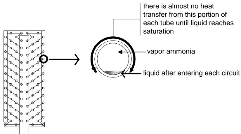
Figure 4: Top-fed evaporator feed with subcooled liquid.
