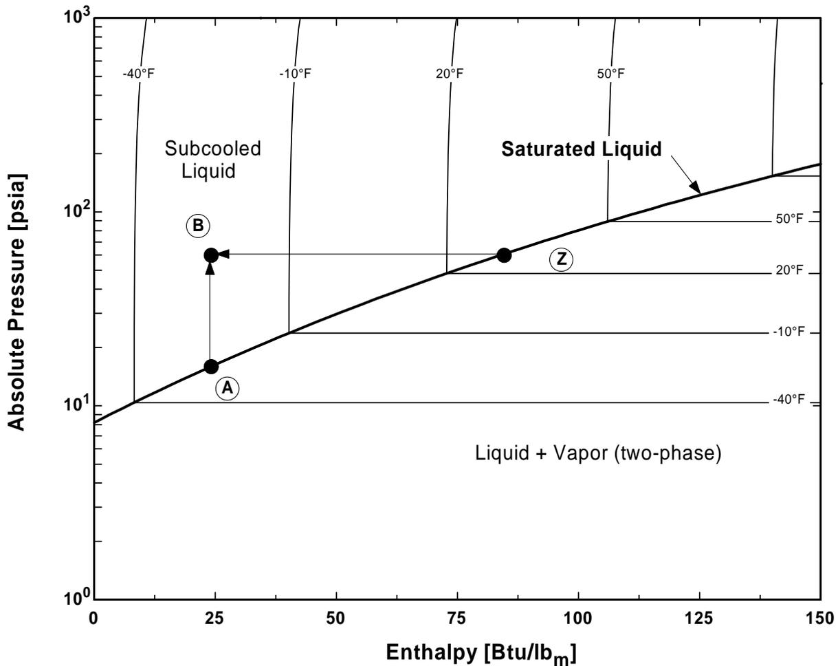
Figure 2: Two ways of subcooling liquid on a p-H diagram.
