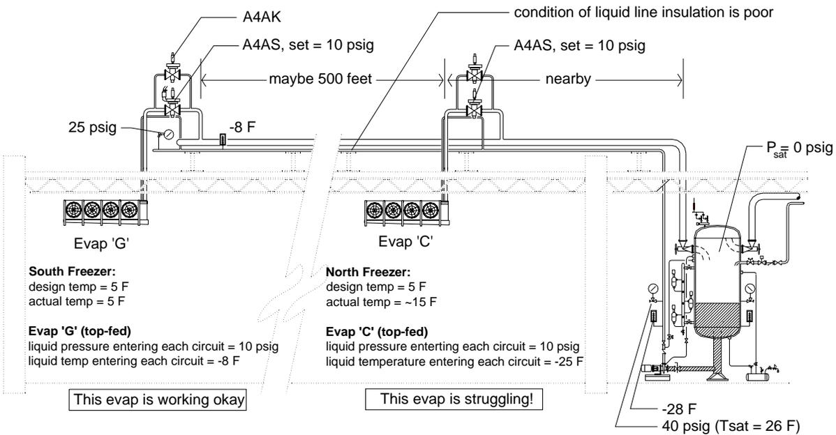
Figure 3 Top-fed evaporators with evaporator pressure regulators
