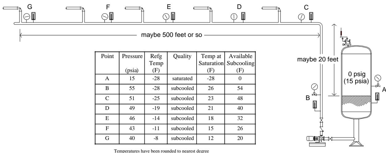
Figure 1: Pumped accumulator & liquid line with defective insulation.
